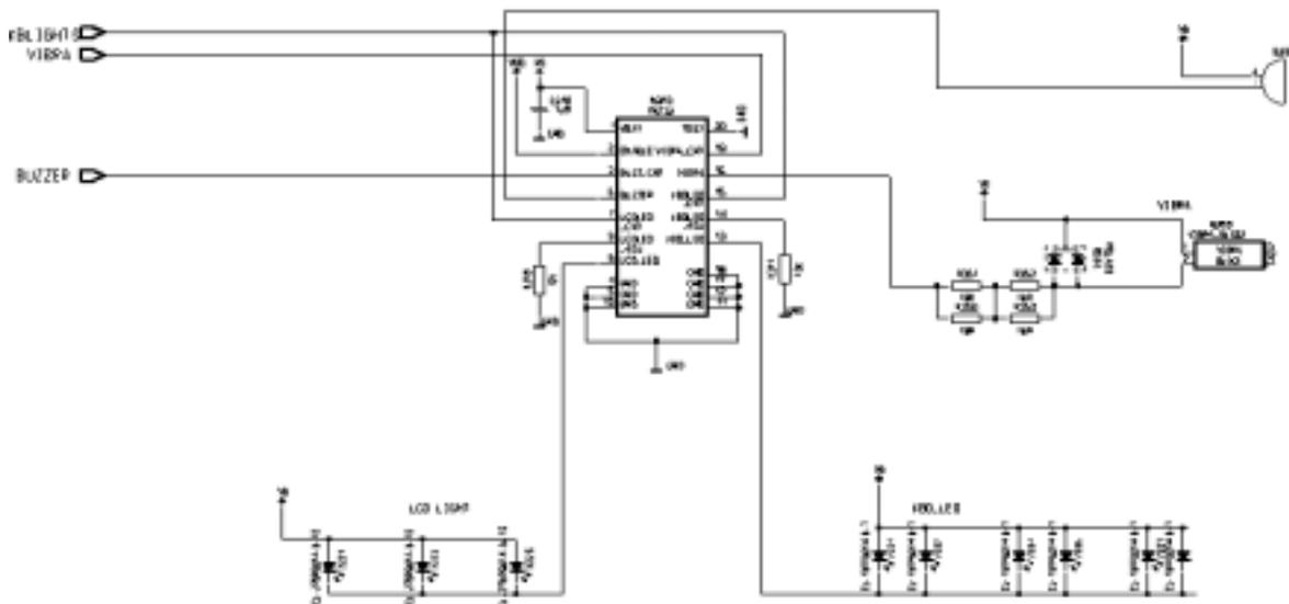
Backlighting is made by LEDs, three LEDs on the bottom of the display. Light is on when LIGHT-signal is in HIGH state.
