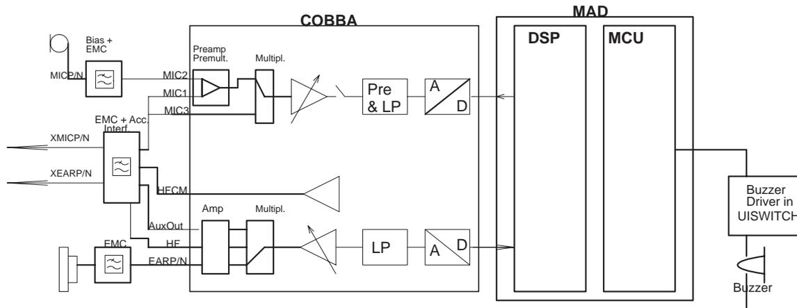
The baseband supports three microphone inputs and two earphone out puts. The inputs can be taken from an internal microphone, a headset microphone or PPH-1 microphones. The microphone signals from different sources are connected to separate inputs at the COBBA-GJP ASIC. In puts for the microphone signals are differential type.
